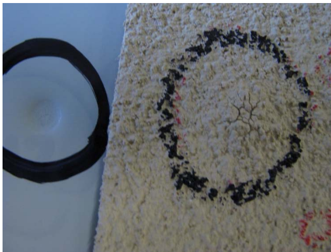
Photo 4: Typical failure when struck from back side of plate (extrusion). Image of indent on the back face is also shown for reference
