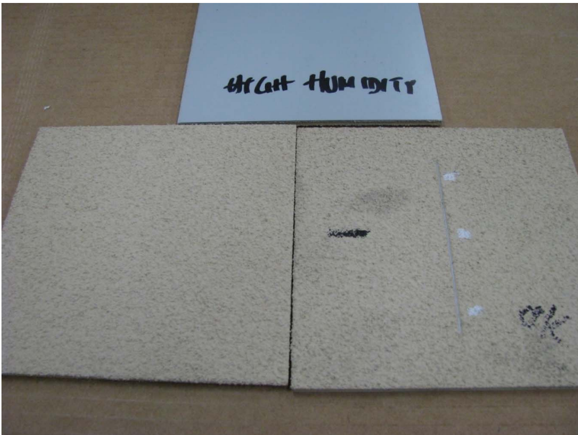
Photo 1: Panels after exposure to high humidity
